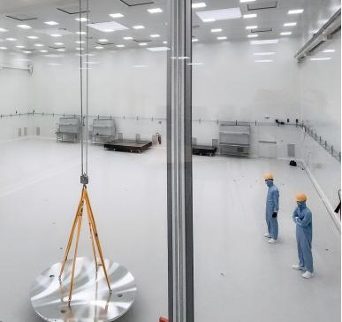
modifications to the experimental setup in terms of load. The flexibility and precision of the two hoists with a load capacity of 4 tonnes will undoubtedly prove useful here. Because when changing the experimental setups and the necessary research equipment that has to be assembled and disassembled, it is mostly unique items that must be connected or separated very precisely and slowly.
